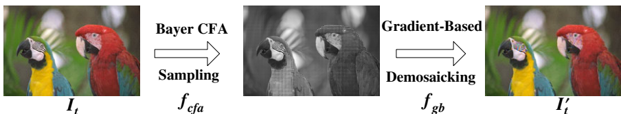
Fig. 4. Flow of the natural counterpart estimation in our method
